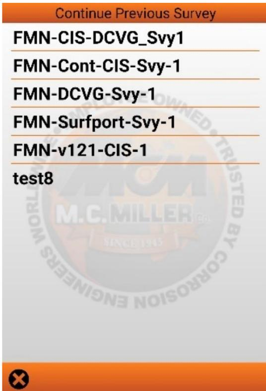
The **Continue Previous** Survey screen lists the surveys on the Android PLS data logger in alphabetical order and allows the user to select a survey to open.
